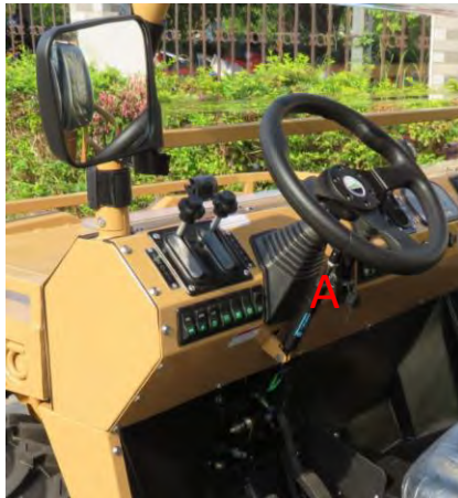
A = Steering column release lever
