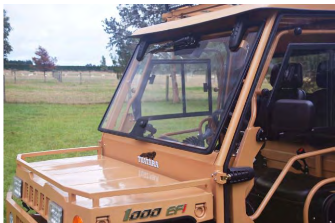
Windscreen in the vented position & with wiper retracted
