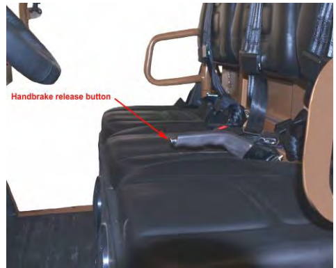
Handbrake in unengaged position
