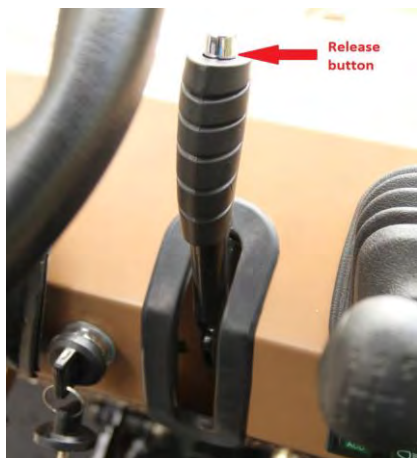
Brake Pedal Lock Lever – Unengaged
