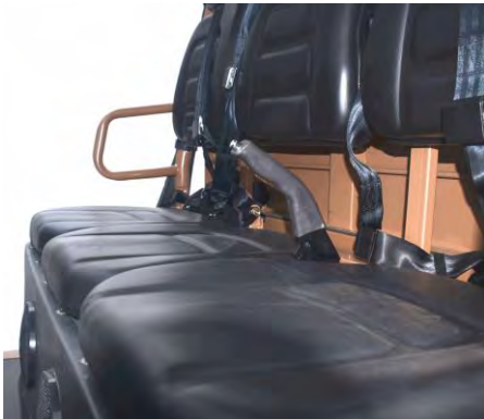
Handbrake in the engaged position
