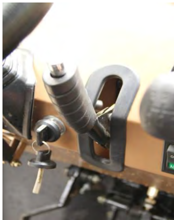
Brake Pedal Lock Lever - Engaged
