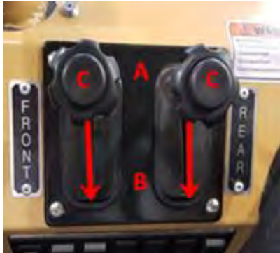
Differential Lock Levers
