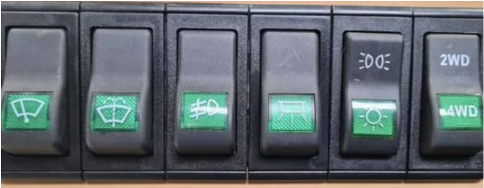
Windscreen Wiper Washer Fog lights Roof light Headlights 2wd / 4wd
