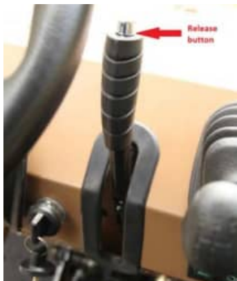
Brake Pedal Lock Lever – Unengaged
